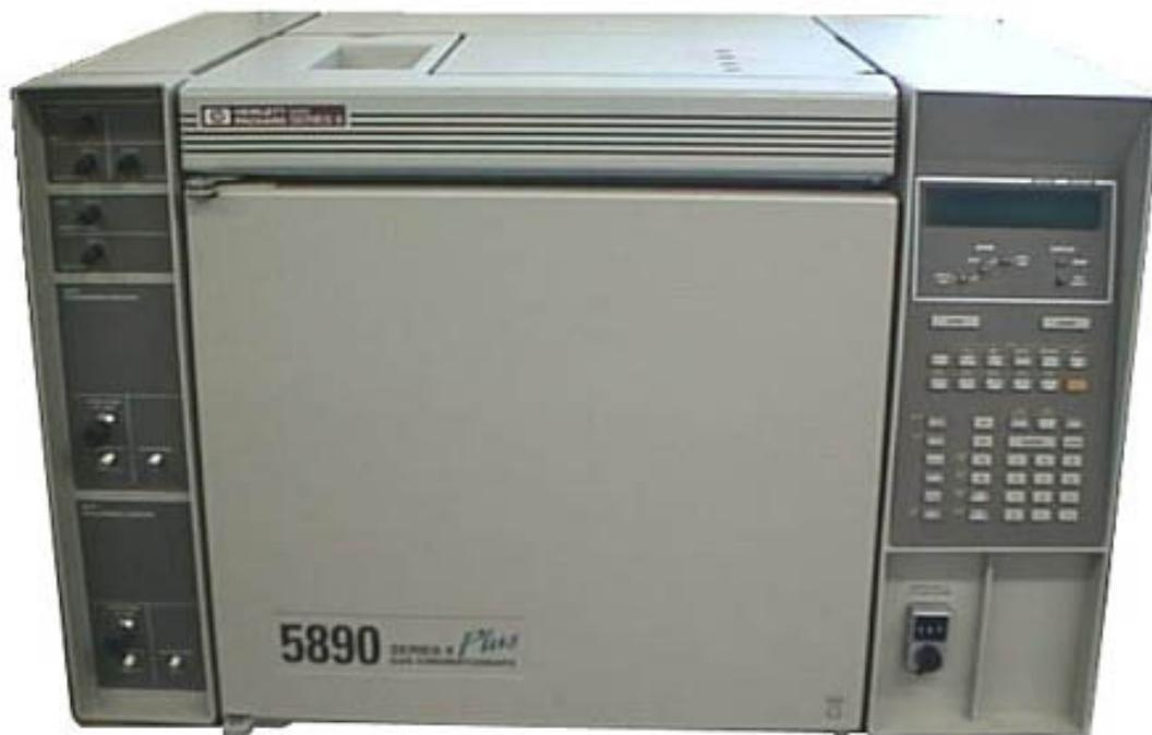
**Fig. 8** Gas-chromatograph HP-5890 Series II.
