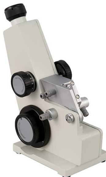
**Fig. 4.** Abbe refractometer.
