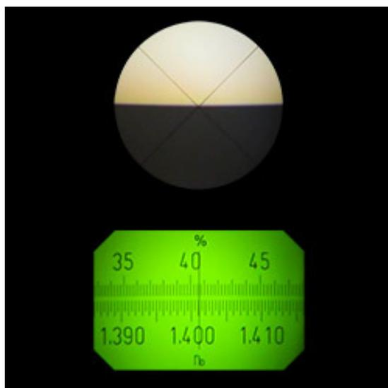
**Fig. 6.** Reading the value of refraction index.
