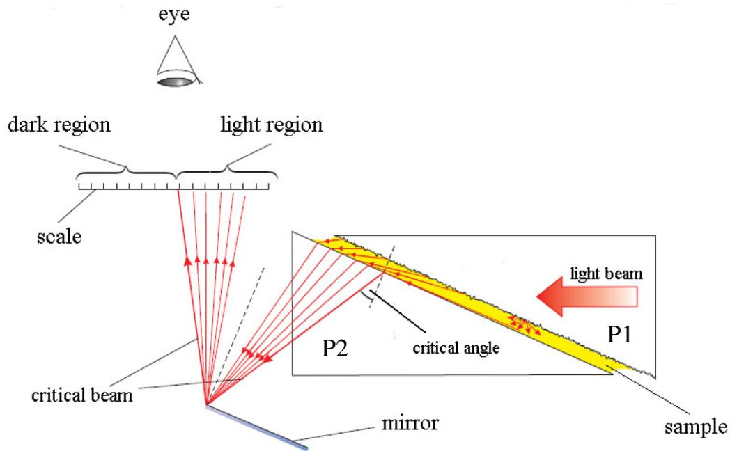
**Fig. 2.** Abbe refractometer - the principle of operation [3].
