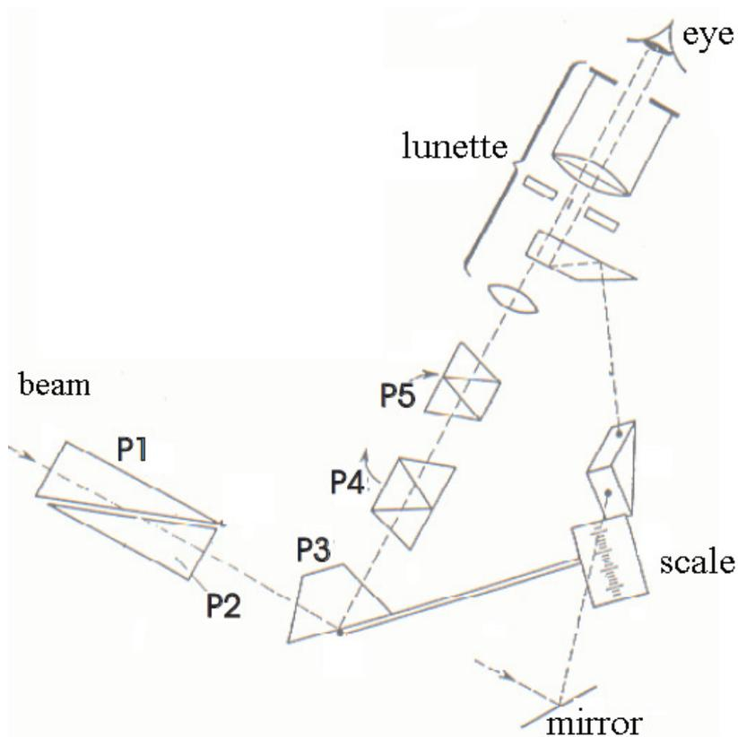
**Fig. 3.** Abbe refractometer – the optical scheme [3].
